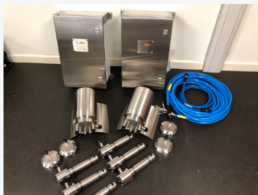
The system comprises three dual axis shear pin load cells, two accelerometers, and a programmable logic controller (PLC).
