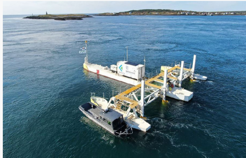
Sustainable Marine's PLAT-I tidal device (Courtesy of Sustainable Marine Energy)
