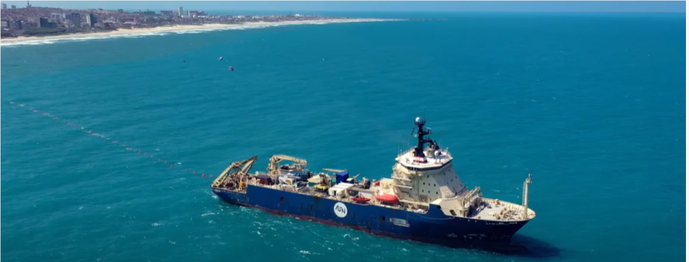
CS "Ile de Brehat" – Shore-end Operation
